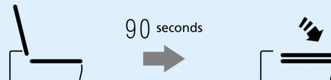
**Under both seat and Lid open :** when the person left the human body sensing range, after 90 seconds, the seat closes automatically. Then, after 80 seconds, the Lid closes automatically.
