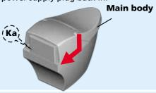
Test FLUSH button to determine if it can be pressed and flush normally. If not, the assembling is not in position. Repeat step 1 to 3 During dismantling the main body, please press SLIDE PLATE button. At the same time, pull the main body 3 cm to the front. Then lift up then dismantle the main body. (During dismantling the main body, pay attention to the dismantling of power supply wiring and water pipe connection.)
